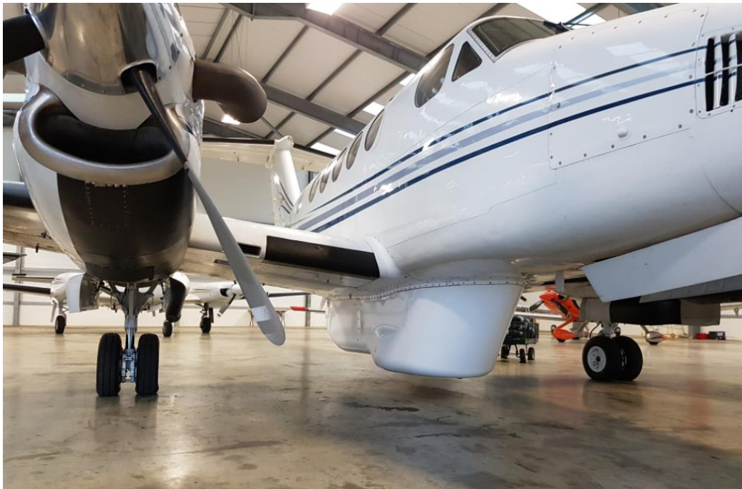
Trials aircraft showing large underbelly radome
